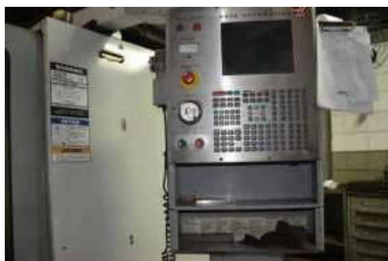
FIGURA 27 - FRESADORA - VOP-B - 30HP - 2-SPEED GEAR DRIVE - 10.000 RPM - TSC THROUGH-SPINDLE - COOLANT
